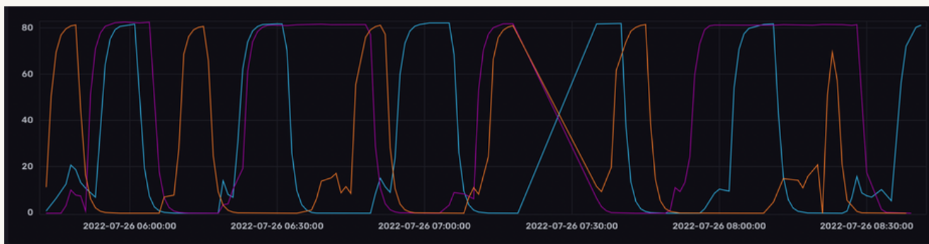
Hash rate in Th/s for the same 3 machines over 3 days with degraded PSUs.
