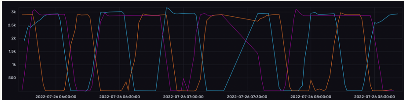
Power consumption in kW for 3 machines over 3 days with degraded PSUs.
