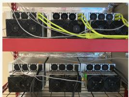
Before exploring the aggregated data, it is also worth noting that given our previous discussion of 4in spacing between vertically mounted machines, 8 machines fit on a single 8ft length of rack. By mounting S19s horizontally and shell to shell, you are able to decrease shelf height from 16in to 10in and subsequently increase rack density by 60%.
