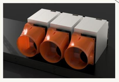
shroud effect is not contingent on a particular firmware suite. Interestingly, the shrouds provide meaningful increases in nominal hash across multiple models of ASIC. Because of the particular shroud design, which exhausts both the PSU and main cooling fans into the same channel, we hypothesize that this attachment allows all unit fans to work together with greater overall efficiency.
